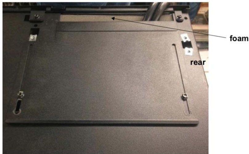
Figure 4: When routing cables directly through the top of the frame, there are two sliding plates on the top of the frame (one on each side of the rear of the frame) that can be opened and any gaps can be eliminated with self-sticking foam. The foam assists with airflow containment. The sliding plates can be used for top exit cabling, even if the Top Exit Cabling feature code is not ordered.
